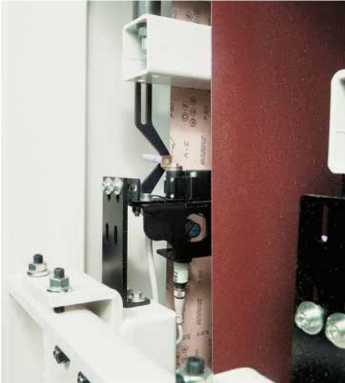
**BELT OSCILLATION CONTROLLED BY AN ELECTRONIC PHOTOCELL**
