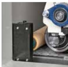
*The out-feed pressure roller allows a uniform and intense pressure in calibrating with high removal and sanding of short and narrow pieces*
