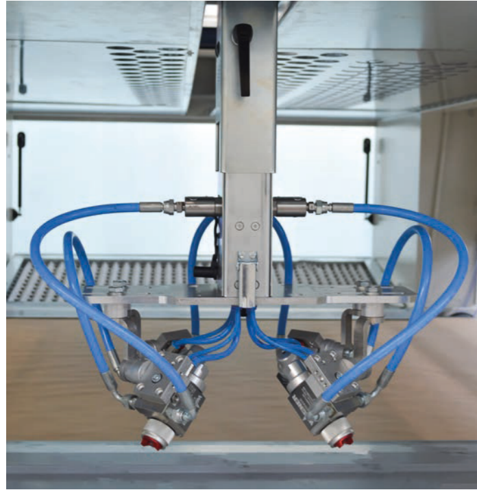
Spraying arm mounted on linear precision guide with brushless motorization, for smooth and precise control of the movement.
