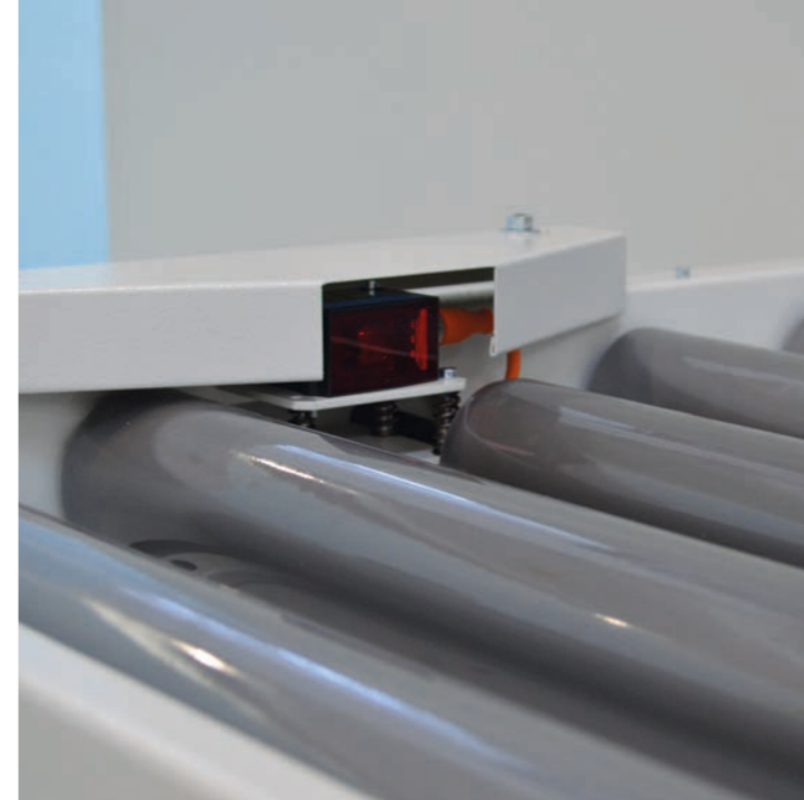
Automatic reading of the working width by laser according to the parts loaded by the operator, allowing optimal management of the opening and closing of the guns to limit the waste of paint.
