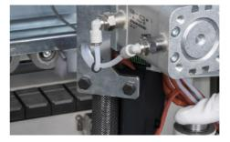
**Ergonomic and accessible**, the glue pot has a quick-release device with the setting for its correct repositioning, which makes the replacement operation quick and without further adjustments.
