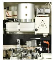
Homogeneous spreading over time thanks to the exclusive glue closing device placed before the roller (SCM patent), and without scrapers that rest on the roller avoiding the problem of the carbonization and the leakage of glue.
