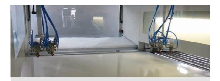
Double reciprocating arm complete with 2 lacquer circuits (a third one can be added as an option). In the standard execution, each arm carries 4 guns. On request it is also possible to have gun holders to carry 6 guns per each arm.
