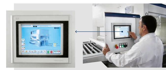
Electronic control via PLC and touch panel; user-friendly software controls the spraying parameters, stores the working recipes, eases diagnostics and programs the ordinary maintenance.
