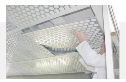
Quick access to the mechanical, electrical parts of the machine without using tools or keys.
