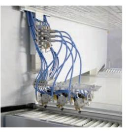
Gun holders, with positions for up to 8 guns each and be used with up to 6 circuits. Options include quick change gun mounting plate assemblies and motorized height adjustment.
