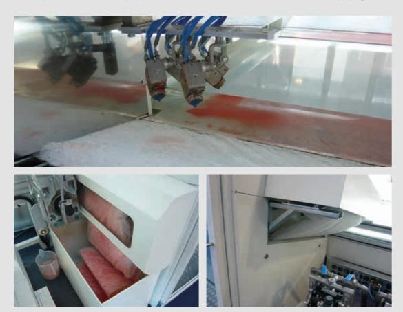
The machine can be supplied with a wet filtering system, particularly utilized in case of high gloss finishing. This system consists of a suction tower with an air scrubber and skimmer for the waste collection. The side filters in the machine are now water "weir" style with continuous water flow to the skimmer for cleaning.
