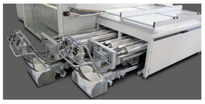
It is possible to install on the machine more units at the same time for an instantaneous quick change and separate lacquer reclaiming of various products.
