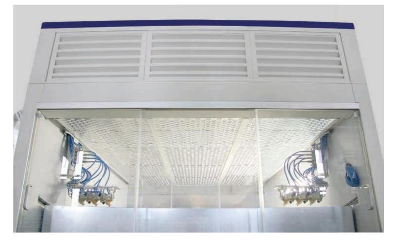
Spray area is supplied with input air from a wide and specially engineered filter roof across the entire spray cabin. It's special design ensures perfectly even air distribution across the full working area. Cabin walls are all fabricated with Stainless steel facings for easy clean up.
