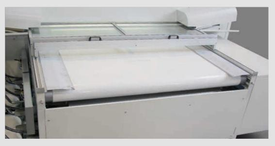
Extra width belt in the spraying area, which achieves a high coating recovery percentage, with less lacquer overspray in the filters. This also prevents the edges of the belt from being contaminated with dried coating.
