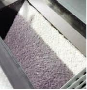
As an alternative to the traditional dry filtering, it is possible to install as option the dry filtering system FILTER ON DEMAND, which automatically changes the filters when needed. The dirty filter automatically changes on operator request or after a certain production has been processed.
