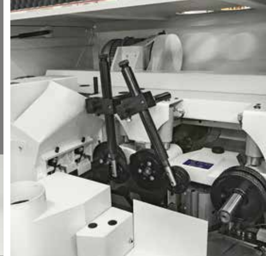
Vertical pressure with idle rollers placed in front of vertical spindles Effective in any situation.
