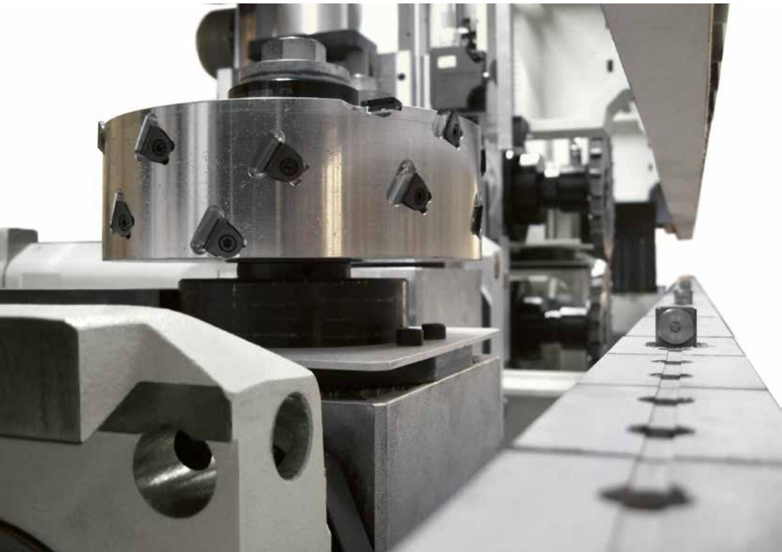
Top pressure beams with spaced pulleys and vertical adjustment according to work piece density, dimensions and profile to always guarantee a precise and uniform movement.
