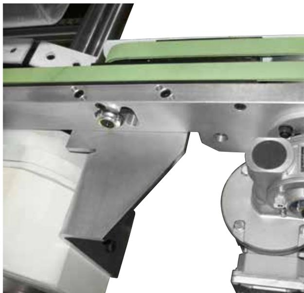
Double belts at machine infeed and/or outfeed with speed regulated by inverter.
