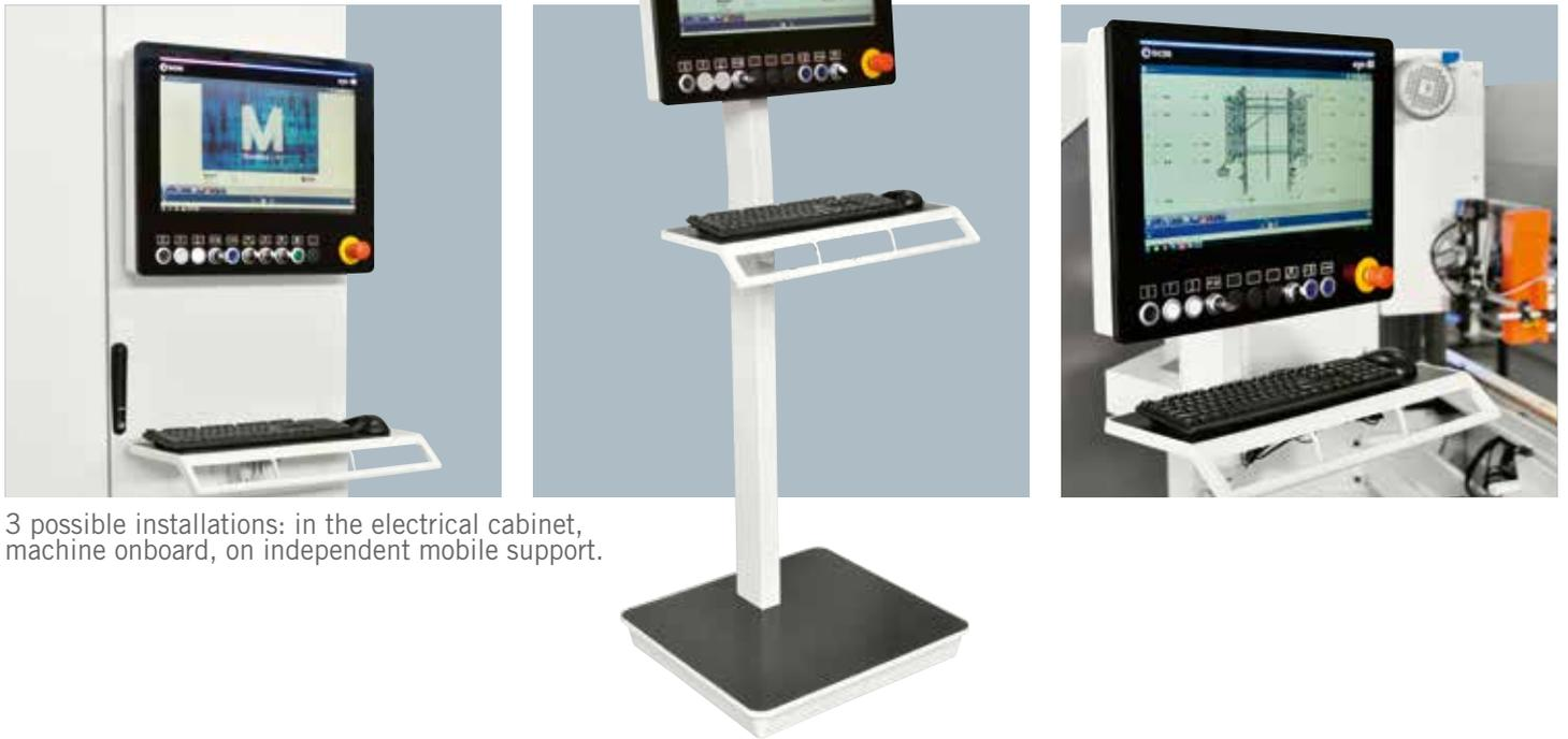
3 possible installations: in the electrical cabinet, machine onboard, on independent mobile support.
