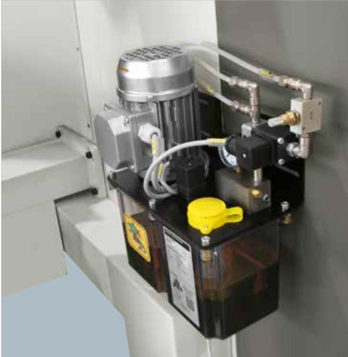
Automatic lubrication system of the guides for the mobile beam positioning, of pressure beams and each brushless axis. It avoids the ordinary manual maintenance of handling machine parts.
