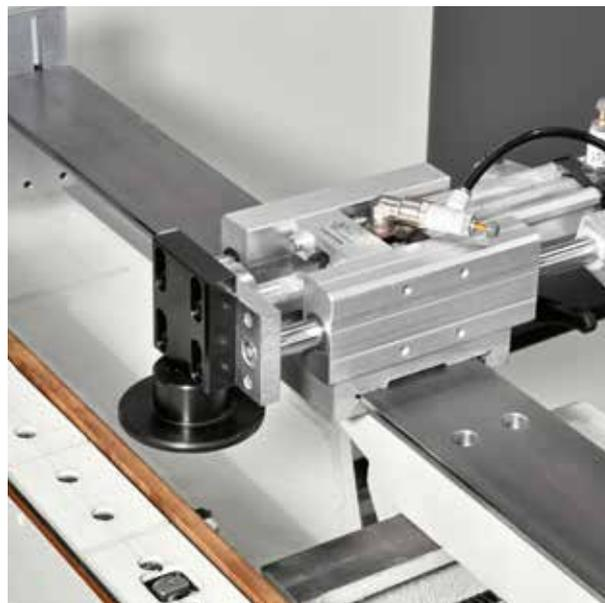
Aligning device to center the panel perfectly.
