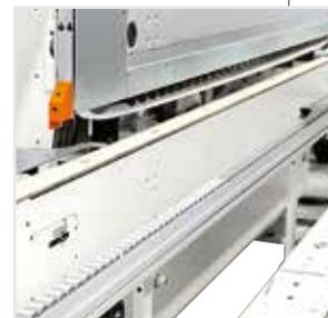
**Adaptability even to larger and more flexible work pieces** thanks to the central, self-centering support with rollers.
