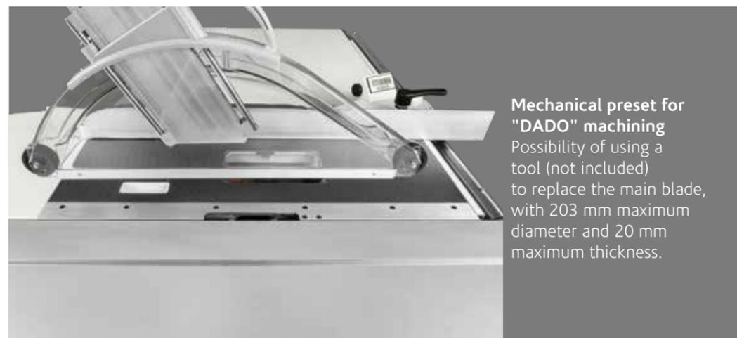
**Mechanical preset for "DADO" machining**
