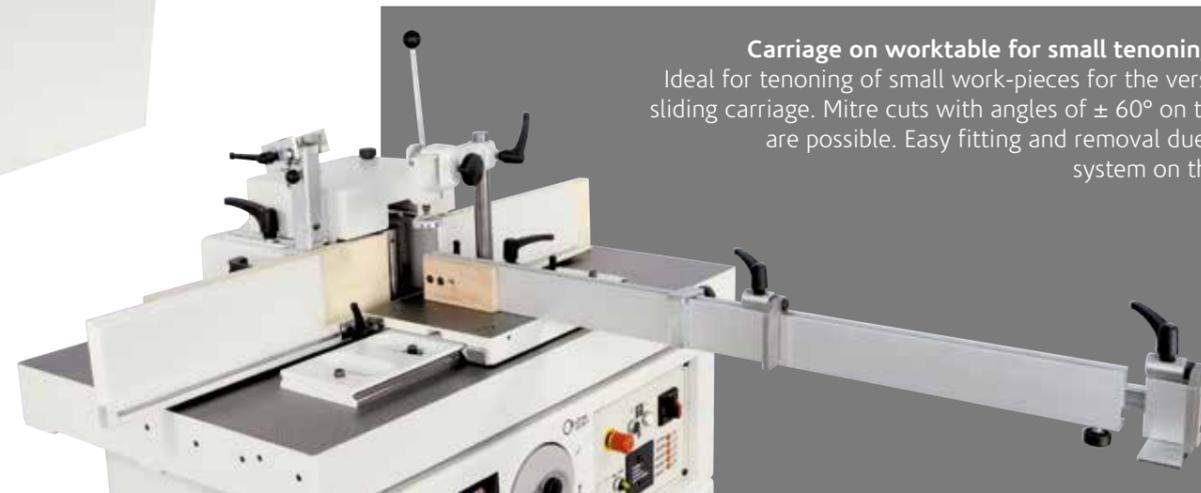
**Carriage on worktable for small tenoning operations**
