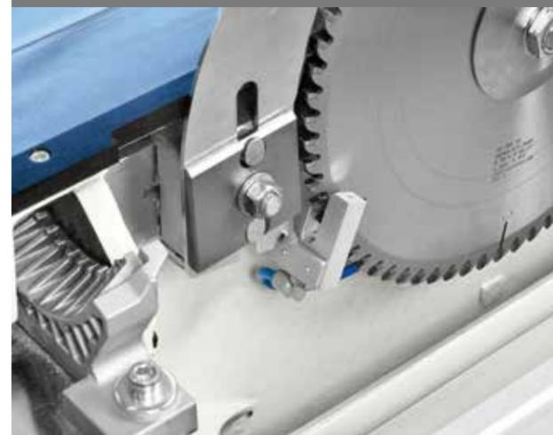
**"LED indicating scoring unit in operation" device**
