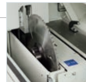
In a few seconds the "SAW-SET" device carries out fast and precise tools adjustment both on cross and longitudinal cutting axes. (opt.)
