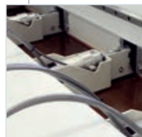
Slotted pressure beam: the best answer for cutting requirements Special openings on the pressure beam eliminate the interference zone with clamps, and greatly reduce the off-cuts.
