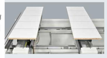
From a single panel can be obtained more elements and automatically re-position them to carry out all machining without interrupting the production cycle; at the end the work pieces are returned to the initial position to facilitate the unloading from the work table.
