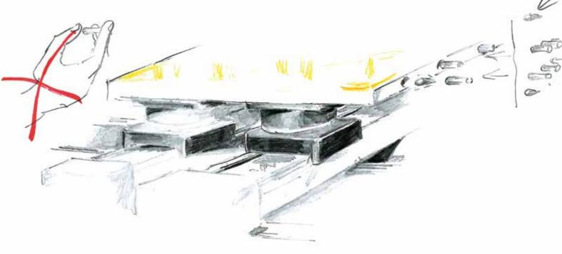
Optimization of productivity with no more time wasting for cleaning operations, thanks to the use of glue capsules, contrary to traditional dowelling devices where it is necessary to remove the remaining drying glue from the various components after a temporary production-stop.
