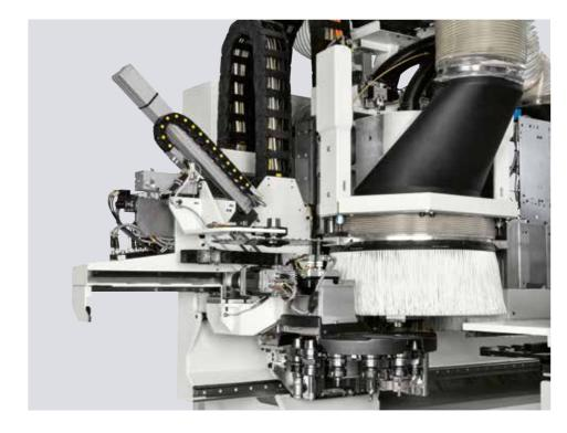
The **"VELOCE" on-board tool changer** with 12 or 16 positions, equipped beside the electrospindle, allows the tool change in hidden time.
