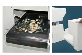
**Rapidity and ergonomics** to equip and do maintenance to the operating group thanks to the practical frontal opening. **No problem with dust or shavings** thanks to the dust shavings conveyor belt equipped with exhaust outlet and the dust collection box located in an ergonomic position.
