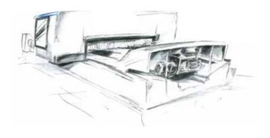
Free access without obstacles on the floor, cable-holder chain and vacuum pump integrated in the machine base.
