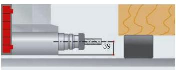
5-axis machining unit geometry allows it to operate at angles of up to 10° below the work piece supporting surface.
