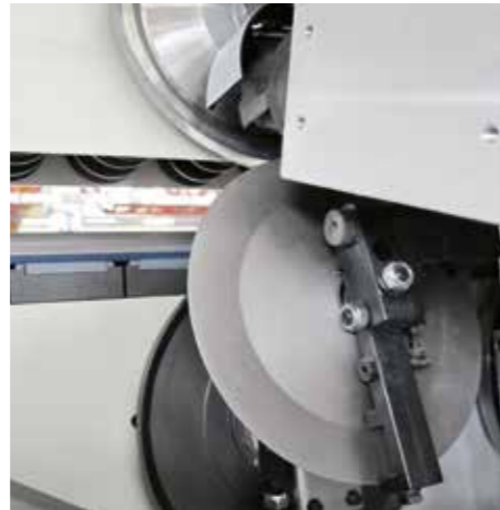
Additional opposite-copying system with large diameter disc. For processing panels with reduced thickness and tendency to bend (opt.)
