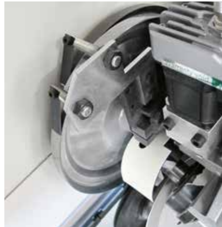
Twin Feeler copying system allowing a constant processing without marks, especially at high speeds (opt.)
