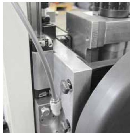
Nesting lock kit instantly stops the vertical copying movement in the presence of nesting holes (opt.)
