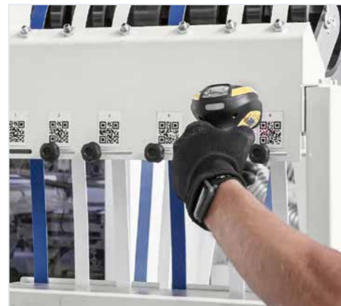
A single database of all the customer's edges, with rapid association of the machining program with the edge used, thanks to the "edge store manager" software. Coding with label and detailed report of the used and remaining edge.
