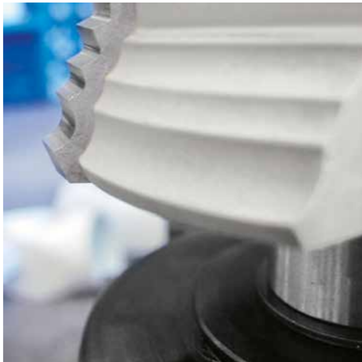
Machining of up to 3 different radii with automatic set up.
