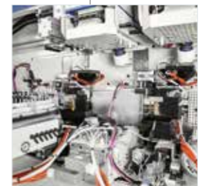
Productive No more machine downtime for glue type and / or color change thanks to the "Glue Switch" system with two integrated glue pots with just in time change.
