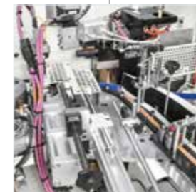
Flexible Magazine for up to 6 edges in rolls with automatic changeover by HMI.
