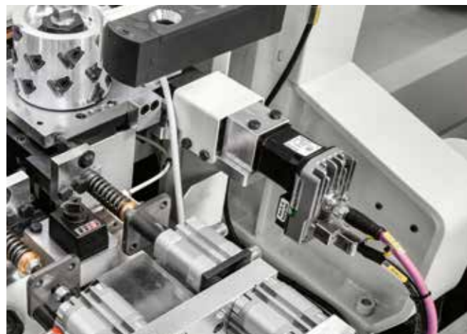
Cutting section set up by HMI with micro-adjustment thanks to NC axis of the first copying device and the entry guide (opt. easy size plus).
