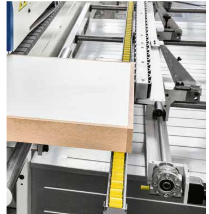
Counter shoulder for narrow panels or solid wood machining (opt).
