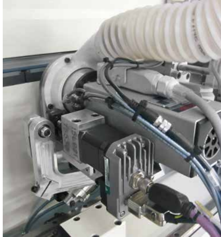
Excellent processing also with change of material or set-up thanks to the microadjustment system of the tool position by HMI. The tool is always in the right processing position.
