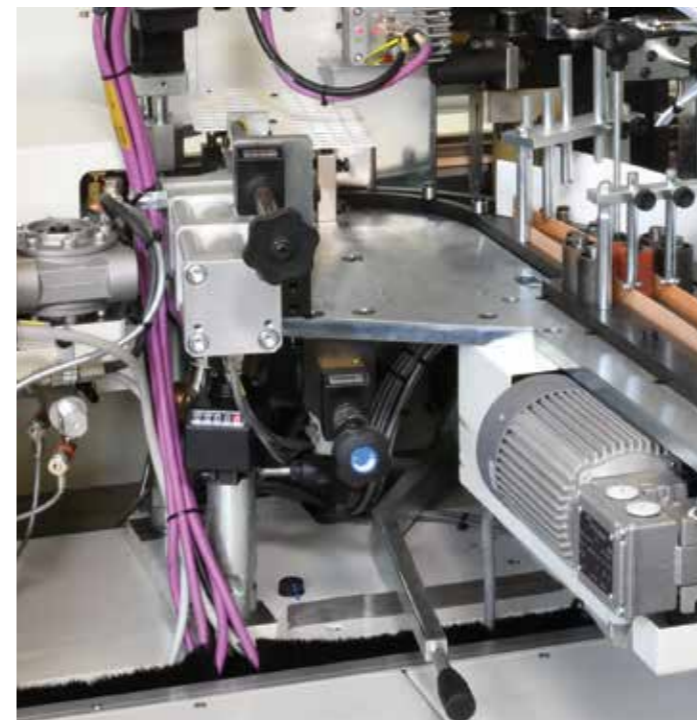
Adjustment of the height of the edge feeding table. It optimizes the edge excess between the upper and lower sides and allows the correct position of any decorations on the edge.
