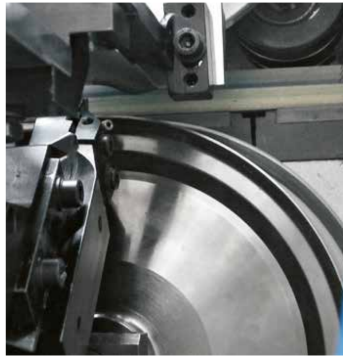
Twin Feeler copying system allowing a constant processing, without marks, especially at high speeds.
