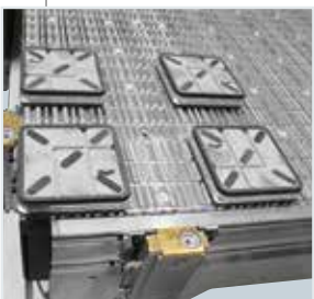
Multifunction worktable suitable for any need of work piece referencing and locking.
