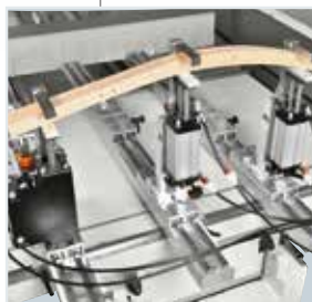
Bars worktable configurable with Combi, Jig free and CSR work piece locking devices.
