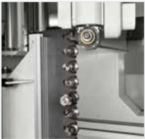
Linear or circular tool store anchored to the upright of the gantry.
