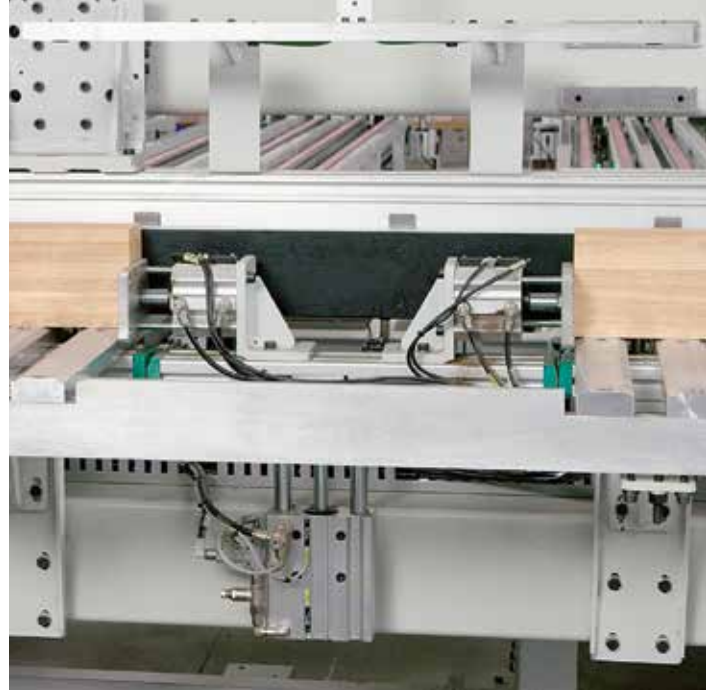
The centering devices ensure the correct work-pieces alignment on the worktable.
