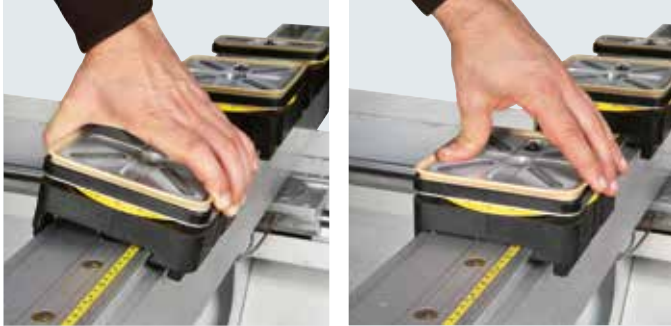
It is possible to add or remove vacuum pods or clamps with a simple movement of the hand; the number and the position are automatically detected.
