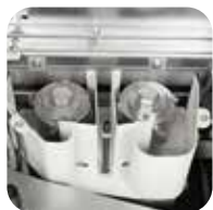
Pre-milling Unit perfect joint line
