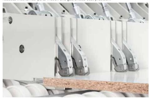
The extreme flexibility of this device is also ensured by the presence of the main pusher grippers, which can be excluded from the working area, so that strips with different widths can be secured and as a result any type of different cutting can be performed without limiting the stroke.
