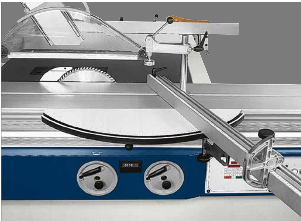
Device for angular cutting with automatic self-adjustment of the stop position with respect to the blade Each time the cutting angle is adjusted so that the distance between the stop and the blade remains constant. This enables rapid set-up and reduces test cutting.
