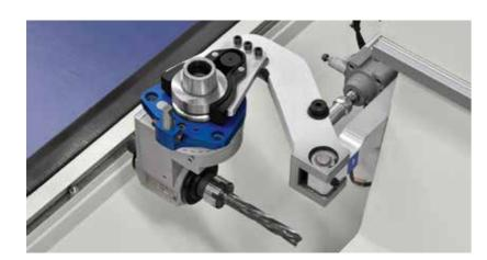
One position "Pick-up" tool changer with pneumatic positioning fitted on the mobile cross beam. Ideal set-up for large sized angular heads.
