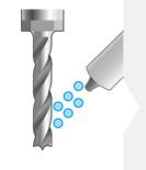
Ionized air blower on electrospindle It is suitable to eliminate the electrostatic charges due to the cut material, making easier the shavings suction (advisable for plastic materials machining).
